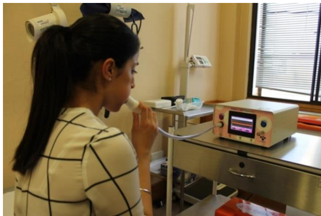
A hydrogen and methane breath test provided by the GastroCH 4 ECK Gastrolyzer
